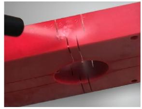
The COMMANDO® XP is an excellent solution for plastics. Dry ice blasting was used to quickly and efficiently deburr the part without causing surface damage.
