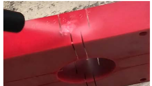
The COMMANDO ® XP is an excellent solution for plastics. Dry ice blasting was used to quickly and efficiently deburr the part without causing surface damage.
